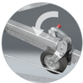
Roue jockey escamotable (ralonge la surface de chargement)
